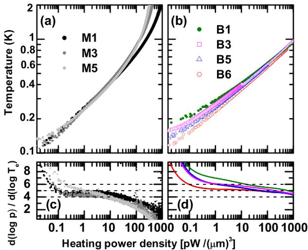
FIG. 4 (color online). (a)  $T_e$  versus  $p = P/V$  for 30 nm membrane samples  $M1$ ,  $M3$ ,  $M5$ . (b)  $T_e$  versus  $p$  for bulk samples, from top to bottom  $B1$  (top),  $B3$ ,  $B5$ , and  $B6$  (bottom). (c)  $d(\log p)/d(\log T_e)$  of the data in (a). (d)  $d(\log p)/d(\log T_e)$  of the data in (b). From top to bottom: green line  $B1$  (top), magenta  $B3$ , blue  $B5$ , Red  $B6$  (bottom). In (d) noise has been filtered to help the eye.
