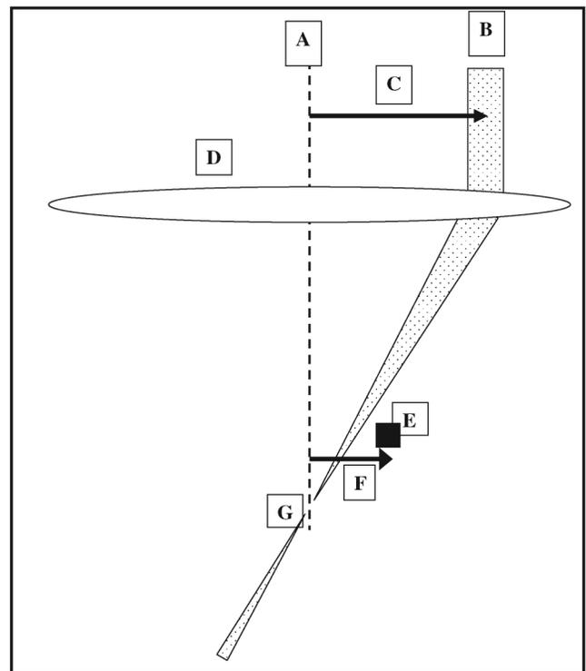
FIG. 2. Main features of the measurements discussed in this Letter. A: Lens optical axis; B: incident pencil beam; C: distance of incident slit center from optical axis which defines the position of the incident pencil beam; D: lens; E: copper fluorescence target; F: detector slit center which defines the distance of the copper target from the optic axis; G: the focal point of the lens.
