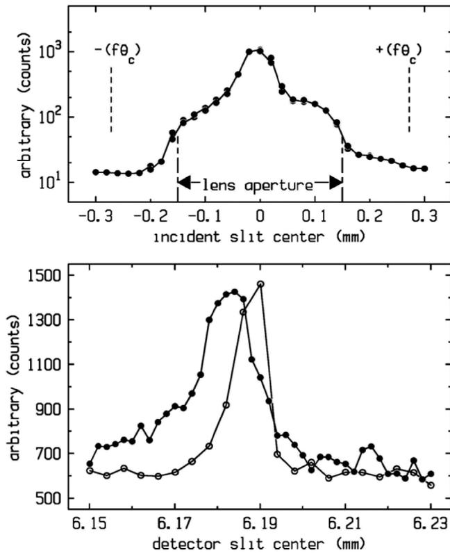
FIG. 3. Top: Scan of incident slit across the lens aperture while monitoring the fluorescence intensity from a lithographically defined target at the focus position. Bottom: Incident slit is fixed near the periphery of the lens, and the Cu target is scanned through the focus. The open circles and the solid circles are two trials with different positions of the incident slit.
