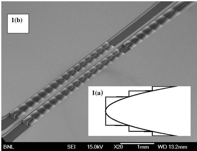
FIG. 1. (a) Inset showing the typical profile of a kinoform structure that results in reduced lens absorption. (b) An electron microscope image of the lenses, showing the single lens in one channel and the first two lenses of the four-lens array.
