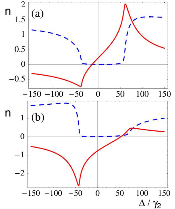
FIG. 3 (color online). Real (solid lines) and imaginary (dashed lines) parts of the refractive index as a function of the probe field detuning  $\Delta$  relative to the radiative decay rate  $\gamma_2$  from level  $|2\rangle$ , for a density of (a)  $N = 5 \times 10^{16} \text{ cm}^{-3}$  and (b)  $N = 5 \times 10^{17} \text{ cm}^{-3}$ .
