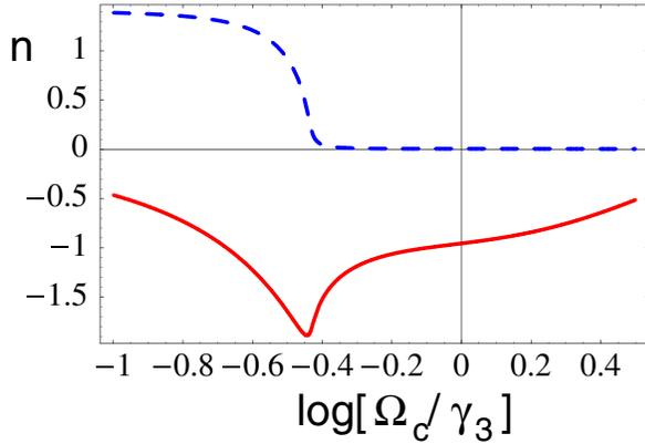
FIG. 5 (color online). Real (solid line) and imaginary (dashed line) parts of the refractive index as a function of the coupling field Rabi frequency  $\Omega_c$  relative to the radiative decay rate  $\gamma_3$ , for  $N = 3.5 \times 10^{17} \text{ cm}^{-3}$  and  $\Delta = -25\gamma_2$ .
