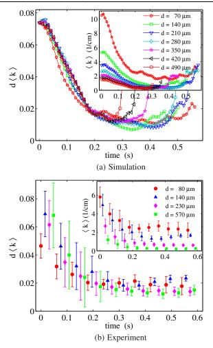
FIG. 4 (color online). Data-collapse plot of  $d\langle k \rangle$  for a series of (a) simulations using glass beads and (b) experiments using polystyrene beads. The grain diameters *d* are given in the legend box. The inset shows the evolution of  $\langle k \rangle$ .
