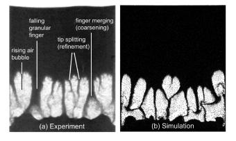
FIG. 1. (a) Experimental image and (b) numerical snapshot of a vertical Hele-Shaw cell where polystyrene beads (in black) of 140  $\mu$ m in diameter displace air (in white). The cells are 56 mm wide and were rotated 0.2 s ago.
