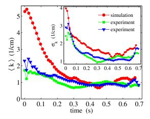
FIG. 3 (color online). Mean wave number  $\langle k \rangle$  and standard deviation  $\sigma_k$  (inset) for two experiments and one simulation, all using polystyrene beads of 140  $\mu$ m in diameter.
