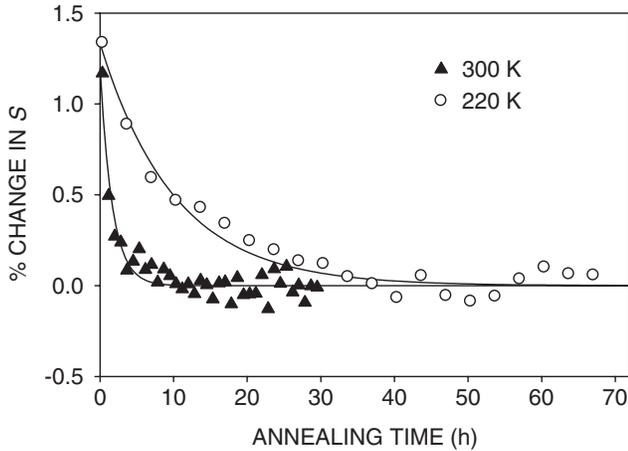
FIG. 3. Percentage difference between the  $S$  parameter for implanted FZ Si (measured at an incident positron energy of 3.5 keV) and its asymptotic value at times  $>3d$  as a function of time at 220 and 300 K.
