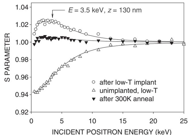
FIG. 2.  $S$  parameter vs incident positron energy for FZ Si at  $25 \text{ K}$ , before and after irradiation with  $\sim 20 \text{ keV}$  He ions, and after annealing at  $300 \text{ K}$ . The solid lines are fits to the data.
