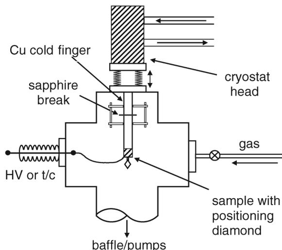
FIG. 1. Schematic diagram of sample chamber.
