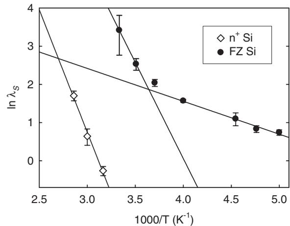
FIG. 5. Arrhenius plots of  $\ln \lambda_S$  vs  $1000/T$ , where  $\lambda_S$  is the decay constant resulting from exponential fits of data such as those in Figs. 3 and 4, and  $T$  is the absolute temperature in K.
