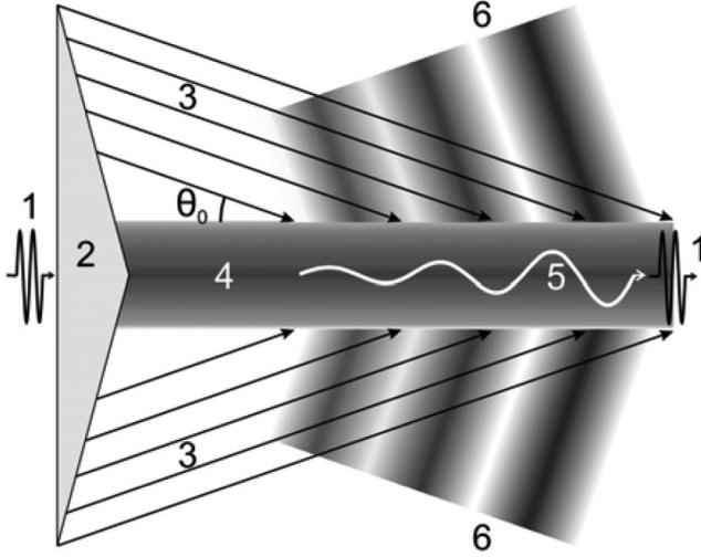
FIG. 1. Schematic of the optical-to-THz wave conversion; 1—laser pulse; 2—axicon lens; 3—refracted rays; 4—pulse-created plasma; 5—laser-field-induced transverse polarization wave; 6—THz radiation fronts.
