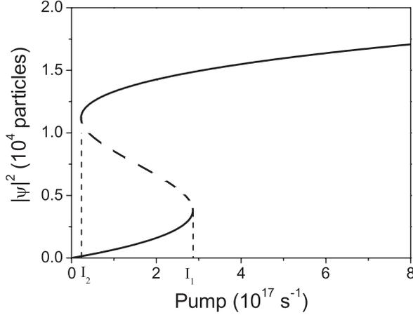
FIG. 1. The polariton population  $|\psi_\sigma|^2$  versus pumping intensity  $|p_\sigma|^2$  for the circularly polarized pump ( $\sigma = \pm 1$ ). Dashed line shows the unstable region.  $I_1$  and  $I_2$  mark two jumps in population caused by the increase and decrease of the pumping intensity, respectively.
