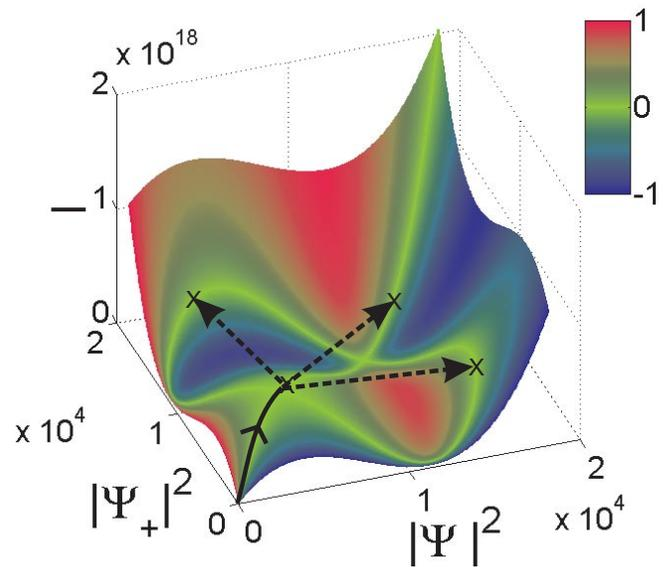
FIG. 3 (color). The pump intensity  $I$  and polarization (color) versus the circular polarized components of the driven mode  $|\psi_{\pm}|^2$ . Color shows the polarization of the pump  $\rho_p$  (bright green corresponds to linear polarization). The crosses mark the four stable points for the driven mode corresponding to the same linearly polarized pump intensity. Arrows show the three possible jumps in case if the pump intensity is slightly increased.
