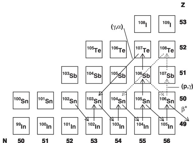
FIG. 1. Portion of the Segrè chart with the path followed by the  $rp$  process in the  $^{100}\text{Sn}$  region as predicted in Ref. [24]. See text for details.
