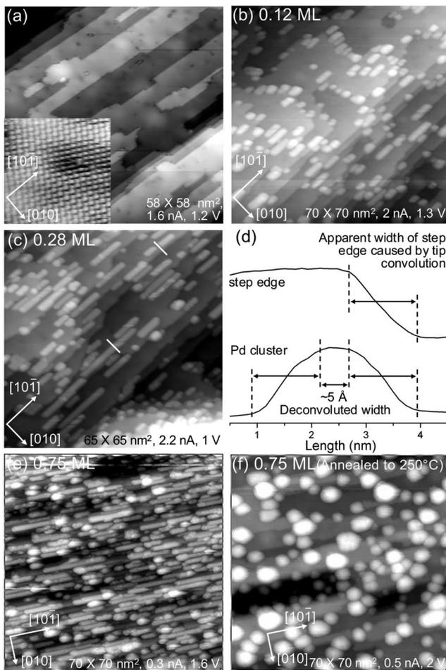
FIG. 2. Empty-states STM images of (a) the clean reduced  $\text{SnO}_2(101)$  surface (inset  $6 \times 6 \text{ nm}^2$ ) and (b), (c), (e) with increasing coverages of Pd deposited at room temperature. Displayed in (d) are line profiles of a step edge and a Pd cluster taken at the positions of the white lines in (c). (f) shows the surface in (e) after annealing.
