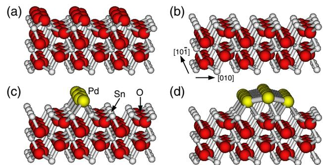
FIG. 1 (color online). Structure of (a) the oxidized, (b) the reduced  $\text{SnO}_2(101)$  surface, and (c), (d) the reduced surface with one and three atom-wide Pd stripes.
