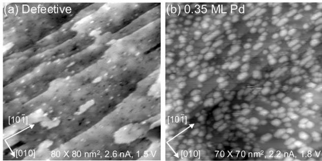
FIG. 4. Constant current STM images of (a) a  $\text{SnO}_2(101)$  surface slightly damaged by  $\text{He}^+$  sputtering and (b) after deposition of 0.35 ML of Pd.
