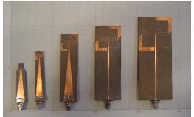
FIG. 2 (color online). Set of near-field resonant antennas.
