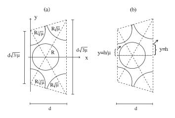
FIG. 2. (a) Geometry of the reference cell. (b) Sketch of the boundary conditions in the periodic cell, as given by Eqs. (1) and (2).
