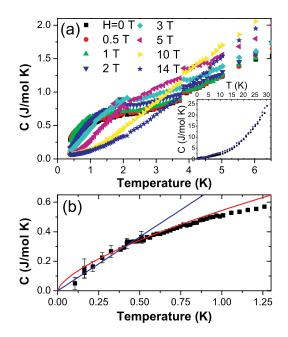
FIG. 2 (color online). (a) The specific heat C(T) of  $ZnCu_3(OH)_6Cl_2$  in various applied fields, measured using a Physical Property Measurement System. Inset: C(T) plotted over a wider temperature range in applied fields of 0 T (square) and 14 T (star). (b) C(T) in zero field measured down to 106 mK. The lines represent power law fits as described in the text.
