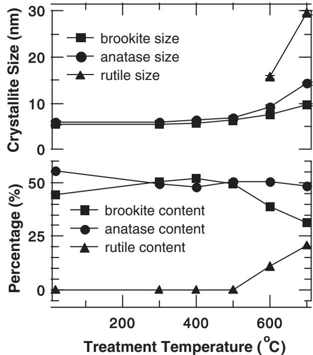
FIG. 3. Crystallite size as a function of treatment temperature (top). Percentage of constituent structures as a function of treatment temperature (bottom).
