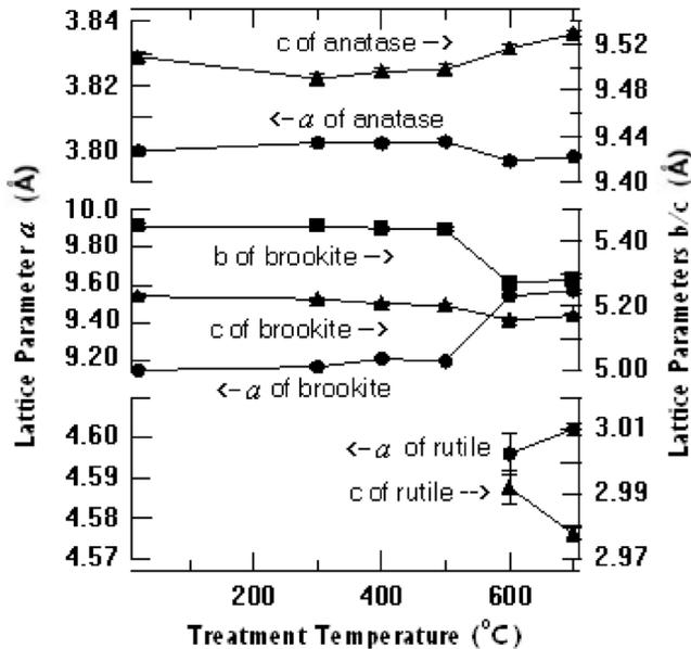
FIG. 2. Lattice parameters of anatase (top), brookite (middle), and rutile (bottom) as a function of treatment temperature.
