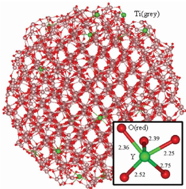
FIG. 1 (color). Distribution of Y atoms (green) at the surface of a 4 nm anatase particle given by a molecular dynamics simulation.
