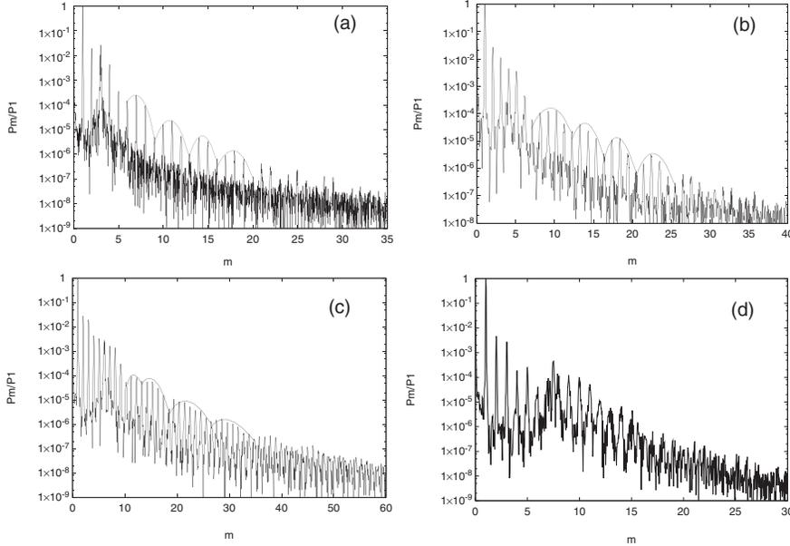
FIG. 2. Harmonic modulation for a laser pulse with  $\tau_p = 17$  fs and  $\lambda_L = 0.248 \mu\text{m}$ : (a)  $a_0 = 0.5$ ,  $n_e/n_c = 10$ , (b)  $a_0 = 0.6$ ,  $n_e/n_c = 19$ , (c)  $a_0 = 1.0$ ,  $n_e/n_c = 40$ , and (d)  $a_0 = 0.5$ ,  $n_e/n_c = 64$ . Envelopes over the harmonics have been added to indicate the respective modulation frequencies.
