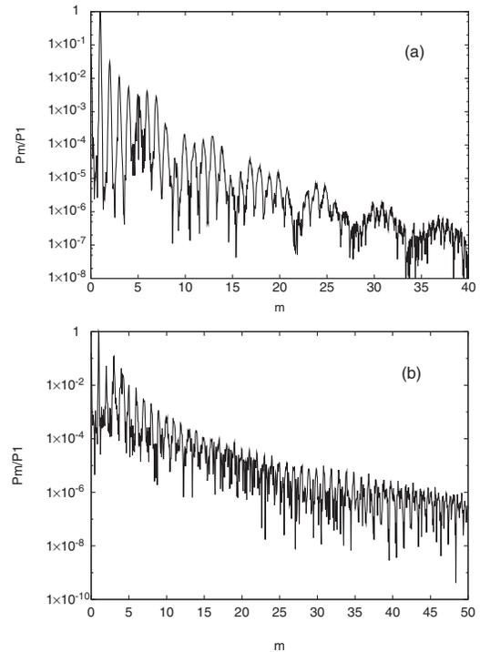
FIG. 3. Harmonic modulation for (a) a laser pulse with  $a_0 = 1.0$ ,  $\tau_p = 30$  fs, and  $n_e/n_c = 30$ , for a steepened pulse envelope; (b) effectiveness of a density ramp in suppressing modulation for a simulation with  $a_0 = 0.6$ ,  $\tau_p = 30$  fs, and  $n_e/n_c = 16$  for a density ramp of width  $\Delta = 0.6\lambda_L$ .
