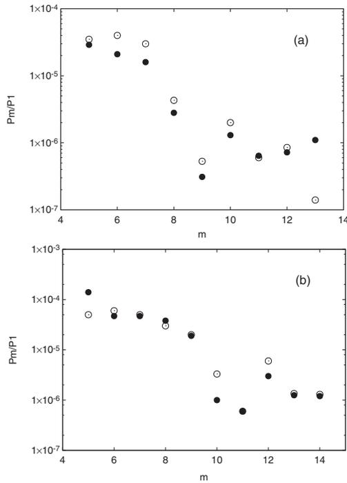
FIG. 4. Harmonic reflected power from PIC simulations and from experiment: (a) solid circles (●) correspond to  $a_0 = 1.0$ ,  $\lambda_L = 0.395 \mu\text{m}$ , and  $n_e/n_c = 30$ ; open circles (○) correspond to emission measured from a carbon target [3]; (b) ●:  $a_0 = 1.0$ ,  $\lambda_L = 0.395 \mu\text{m}$ ,  $n_e/n_c = 45$ , and  $\tau_p = 17 \text{ fs}$ ; ○: correspond to emission found from a glass target [3].
