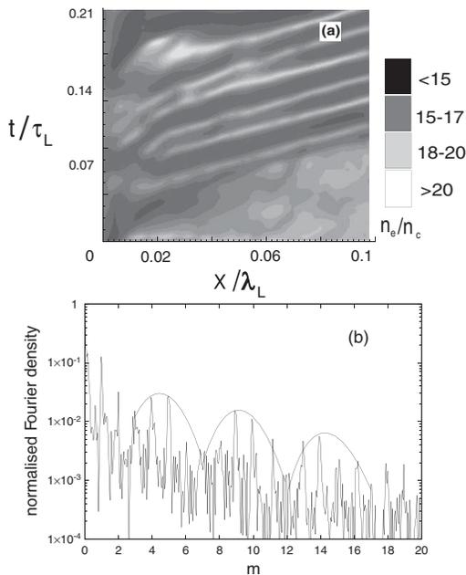
FIG. 1. (a) Plasma electron density contours for a target plasma density  $n_e/n_c = 20$ ,  $a_0 = 0.5$ , with angle of incidence  $\theta = 23^\circ$ . The time scale corresponds to 3 laser periods,  $\tau_L$ , and the section of plasma shown extends over  $0.1\lambda_L$ . (b) Fourier decomposition of the electron density at a point  $x = 0.1\lambda_L$  inside the plasma.
