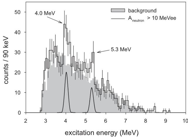
FIG. 2. Reconstructed excitation energy spectrum of  $^{23}\text{O}$ .  $A_{\text{neutron}} > 10$  MeVee. Shaded spectrum represents the background (see text). In order to purify the spectrum, the neutron TOF was confined between 25 and 48 ns corresponding to a range of  $13 \text{ MeV} < E_{\text{neutron}} < 53 \text{ MeV}$ .
