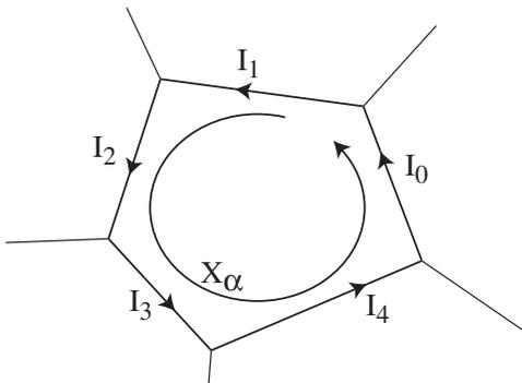
FIG. 1. Sketch of a loop  $\alpha$  indicating the direction of the currents. Every perturbation of the  $I_{kl}$  satisfying the constraints can be written as a weighted sum of such loops.
