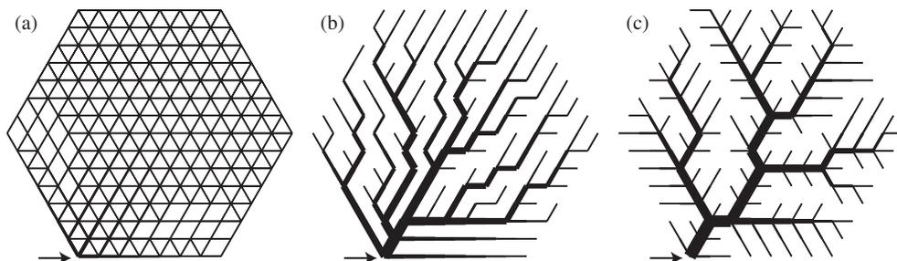
FIG. 2. Examples of the optimized conductivity distributions obtained by the relaxation method for (a)  $\gamma = 2.0$  and (b)  $\gamma = 0.5$ . For  $\gamma < 1$ , the relaxation leads in general only to a local minimum. The global minimum can be approached by searching in the space of tree topologies. The result for  $\gamma = 0.5$  is shown in (c). The arrows indicate the localized inlet.
