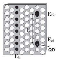
FIG. 1. Simple schematic showing indirect coupling between two photonic crystal cavities connected through an integrated waveguide. Cavity 1 contains an embedded QD. The propagating Bloch mode is labeled as  $\mathbf{E}_k$ , while the cavity modes are  $\mathbf{E}_{c1}$ and  $\mathbf{E}_{c2}$ , that are spatially separated by *L*.
