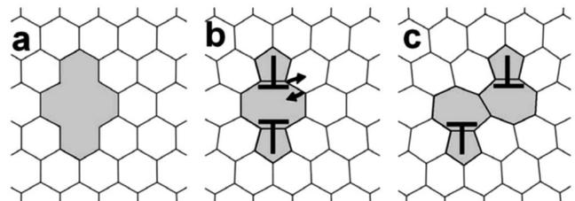
FIG. 2. Removal of two atoms creates a divacancy (a), (b), and can also be viewed as a removal of a small segment of a full crystal plane, leaving the two extra planes, that is two edge dislocations (b) able to glide away (b  $\rightarrow$  c).
