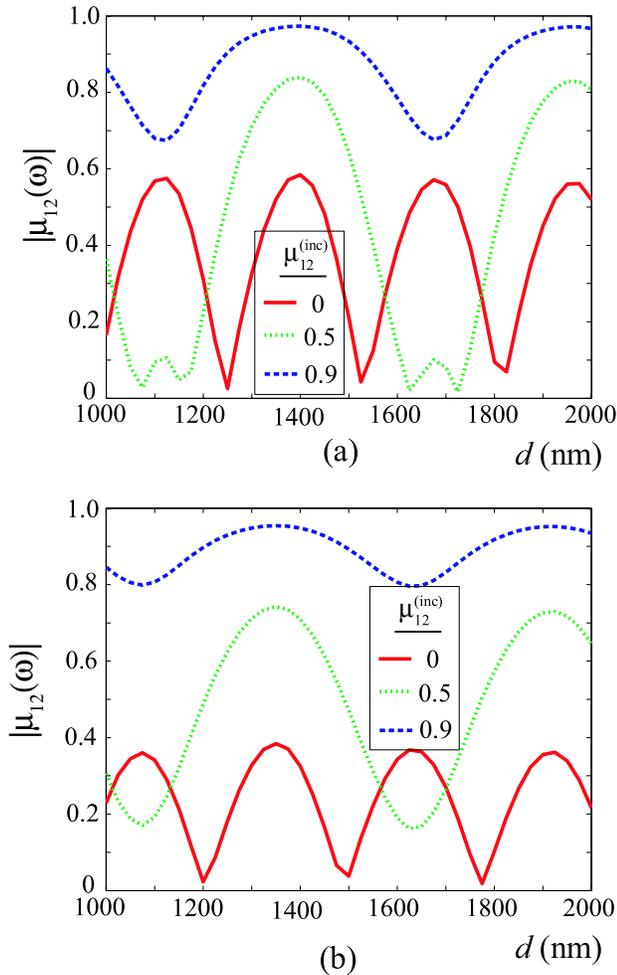
FIG. 3 (color online). The absolute value of the spectral degree of coherence  $|\mu_{12}(\omega)|$  as a function of  $\mu_{12}^{(\text{inc})}(\omega)$ , for slit widths: (a)  $w = 100$  nm, (b)  $w = 50$  nm. For the sake of clarity, only numeric results are shown.
