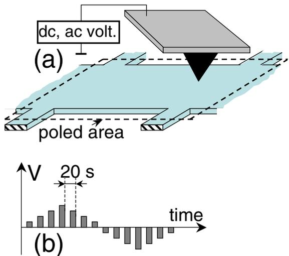
FIG. 1 (color online). (a) Sketch showing the poling or measuring procedure for the Hall bar prepared on  $(\text{Cd}, \text{Zn})\text{Te}/\text{CdTe}$  quantum well for study of nonvolatile gate effect. (b) Voltage profile used for  $d_{33}$  loop measurements.
