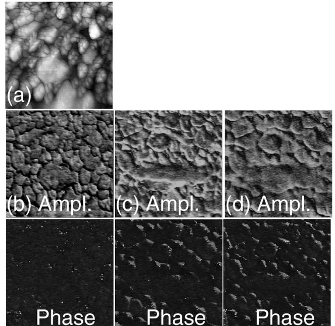
FIG. 3.  $2 \times 2 \mu\text{m}$  topography image (a) and maps of amplitude and phase of local piezoelectric response measured on (Cd,Zn)Te polycrystalline film (b)–(d). Image (b) was taken before poling, image (c) after poling with +15 V at 1 h delay, and image (d) at 24 h delay.
