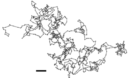
FIG. 2. Trajectory of a single \text{SiO}_2 sphere with s \approx 0.8 \mu\text{m} radius [13]. The trajectory consists of 1024 measurements (black points) and spans a total of 2.2 s. The scale bar indicates 10 \mu\text{m} .
