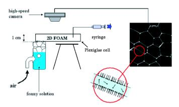
FIG. 2 (color online). Experimental setup: a two-dimensional foam is created in a 1 cm high horizontal Plexiglas cell by blowing air through a surfactant solution. The bubbles are polyhedral with an edge length of 1–2 cm and the liquid fraction in the foam is about 1%. Using a syringe, air is blown away from one bubble, which induces rearrangements, that are viewed from above using a high-speed camera.
