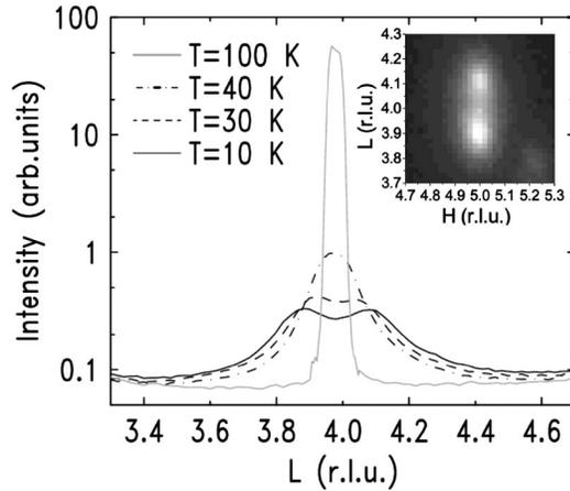
FIG. 2. X-ray scans at the (5, 5, 4)  $F$  peak position at various temperatures. The data were taken on warming from  $T_{\text{irr}} = 10$  K as described in the text. The inset shows x-ray diffuse scattering pattern in the vicinity of this position at  $T = 10$  K. The units for  $H$  and  $L$  are reciprocal lattice units (r.l.u.)
