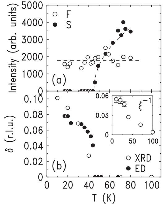
FIG. 3. Temperature dependence of (a) the integrated intensities of the forbidden ( $F$ ) and the superlattice ( $S$ ) peaks from ED measurements. (b) Displacement of the scattering maxima from the positions of the commensurate  $F$  peaks (the incommensurability of the  $c$ -axis lattice modulation) from XRD and ED data. The inset shows the  $c$ -axis inverse correlation length of the diffuse peaks from XRD data, in  $\text{\AA}^{-1}$ .
