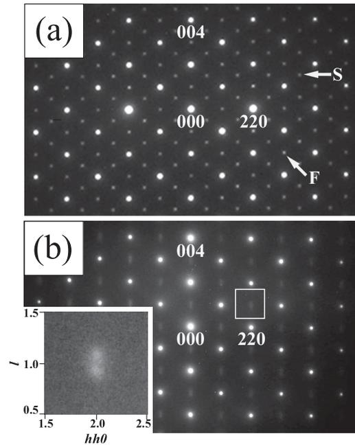
FIG. 1. Electron diffraction patterns for (a)  $T = T_{\text{irr}} = 93$  K and (b)  $T = T_{\text{irr}} = 19$  K. The incident beam is parallel to the [1-10] cubic axis. The inset in (b) shows the enlargement of the diffraction pattern in the vicinity of the  $(2, 2, 1)$  position at  $T = 19$  K.
