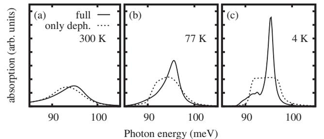
FIG. 3. Absorption spectra with  $e$ -ph interaction in a GaAs QW with a carrier density of  $1.2 \times 10^{12} \text{ cm}^{-2}$ , considering the full dynamics (solid) and with dephasing only (dashed) at a temperature of (a) 300, (b) 77, and (c) 4 K.
