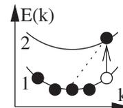
FIG. 1. Band structure of a two subband system in a QW. Optical ISB transition from subband 1 to subband 2. The dashed line illustrates the Coulomb interaction between electrons in different subbands.
