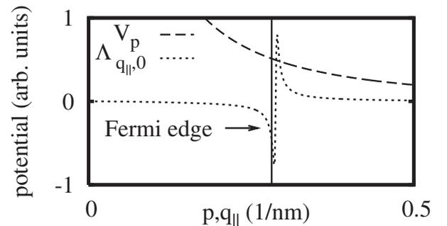
FIG. 2. Comparison of  $V_{\mathbf{p}}^{2121}$  and  $\Lambda_{\mathbf{q}_{\parallel}, 0}^{1221}$ , for a 10 nm wide GaAs QW. Fermi edge—for a carrier density of  $1.2 \times 10^{12} \text{ cm}^{-2}$ .
