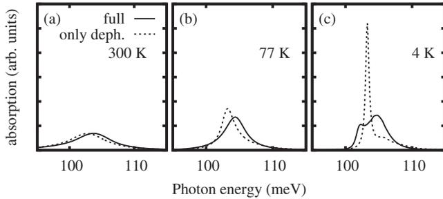
FIG. 4. Absorption spectra with  $e$ -ph and  $e$ - $e$  interaction in a GaAs QW with a carrier density of  $1.2 \times 10^{12} \text{ cm}^{-2}$ . Considering the full dynamics (solid), with dephasing for the phonons only (dashed). (a) 300, (b) 77, and (c) 4 K.
