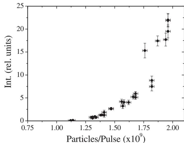
FIG. 2. Demonstration of the threshold behavior of the laser.
