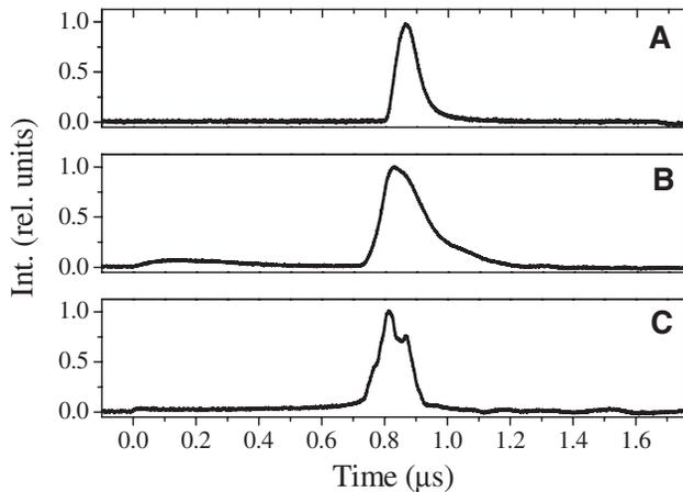
FIG. 3. Time structure of laser emission (a), spontaneous emission (b) and ion-beam pulse (c). The time structure of the ion-beam intensity was measured with an inductive current probe.
