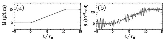
FIG. 1. (a) Typical driving torque applied to the oscillator. (b) Response of the oscillator to the external torque (gray line). The dark line represents the mean response  $\bar{\theta}(t)$  to the applied torque  $M(t)$ .
