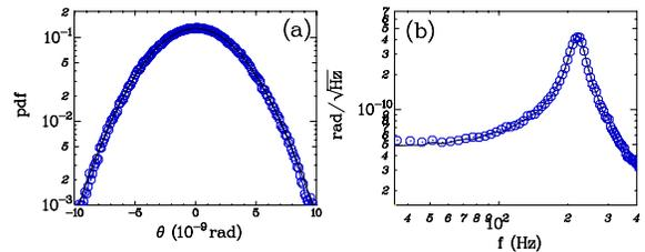
FIG. 5 (color online). (a) PDF of the fluctuations  $\delta\theta = \theta - \bar{\theta}(t)$  when the torque is applied ( $\circ$ ), compared with a Gaussian fit of the PDF at equilibrium (continuous line). (b) The measured spectrum of  $\delta\theta$  ( $\circ$ ) is compared with the prediction of fluctuation dissipation theorem in equilibrium (continuous line).
