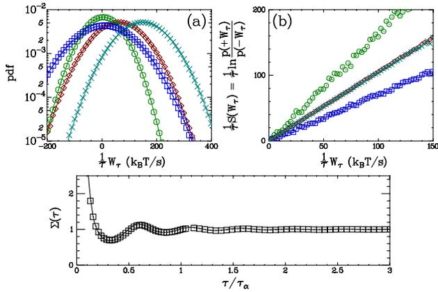
FIG. 3 (color online). SSFT with a ramp forcing. (a) PDF of  $W_\tau$  for various  $\tau/\tau_\alpha$ : 0.019 ( $\circ$ ), 0.31 ( $\square$ ), 2.09 ( $\diamond$ ), and 4.97 ( $\times$ ). (b) Corresponding functions  $S(W_\tau)$ . (c) The slope  $\Sigma(\tau)$  of  $S(W_\tau)$  is plotted versus  $\tau$  [ $\square$ : experimental values; continuous line: theoretical prediction Eq. (10) with no adjustable parameter].
