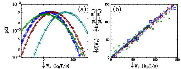
FIG. 2 (color online). TFT. (a)  $P(W_\tau)$  for TFT for various  $\tau/\tau_\alpha$ : 0.31 ( $\circ$ ), 1.015 ( $\square$ ), 2.09 ( $\diamond$ ), and 4.97 ( $\times$ ). Continuous lines are Gaussian fits. (b) TFT;  $S(W_\tau)$  computed with the PDF of (a). The straight continuous lines are fits with slope 1, i.e.,  $\Sigma(\tau) = 1, \forall \tau$ .
