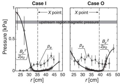
FIG. 5. Radial profiles of axial magnetic field pressure (circles) and electron thermal pressure (squares) measured on the mid-plane ( $z = 0$ ) in cases I (left) and O (right) counterhelicity merging.
