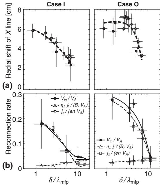
FIG. 4. Radial shift of the  $X$  line (a) and total reconnection rate (solid circle), resistive diffusion term (open triangle), and the Hall term (open square) in the generalized Ohm law (b) as functions of collisionality parameter in cases I (left) and O (right) counterhelicity merging. The curves are approximating polynomials.
