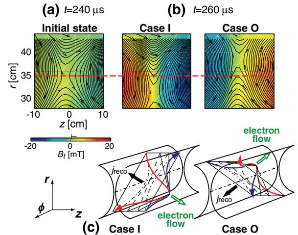
FIG. 3 (color). Measured poloidal magnetic flux contours (solid lines) with poloidal magnetic field (arrows) and toroidal magnetic field (color coded) at  $t = 240 \mu\text{s}$  (a) and  $t = 260 \mu\text{s}$  (b) in cases I (left) and O (right) counterhelicity merging, and corresponding three-dimensional illustrations of reconnecting field lines in the Hall-MHD regime (c).
