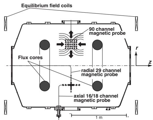
FIG. 1. Schematic view of MRX experimental setup. Arrows indicate plasma inflow and outflow directions to/from the  $X$  line in counterhelicity merging experiments.
