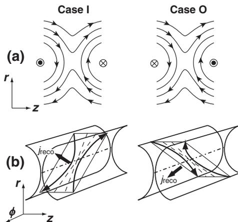
FIG. 2. Two-dimensional (a) and three-dimensional (b) illustrations of reconnecting magnetic field lines in cases I (left) and O (right) counterhelicity merging in the MHD regime. The reconnection current  $j_{\text{reco}}$  has opposite radial components in cases I and O.
