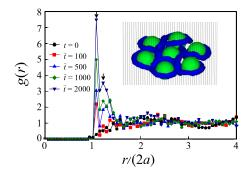
FIG. 3 (color online). Time development of g(r). The inset shows a sheetlike planar aggregated structure composed of seven particles bound by a single-stroke defect loop.
