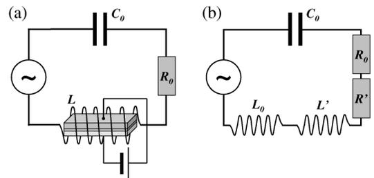
FIG. 4. (a) Resonant RLC circuit for the spin-injection maser connected to a rf voltage source. The paramagnetic medium is enclosed within the inductor coil (the bare coil has inductance  $L_0$ ). The modification of the inductance by the complex magnetic susceptibility of the paramagnet results in the equivalent circuit (b), with an additional resistance  $R'$  and inductance  $L'$ .
