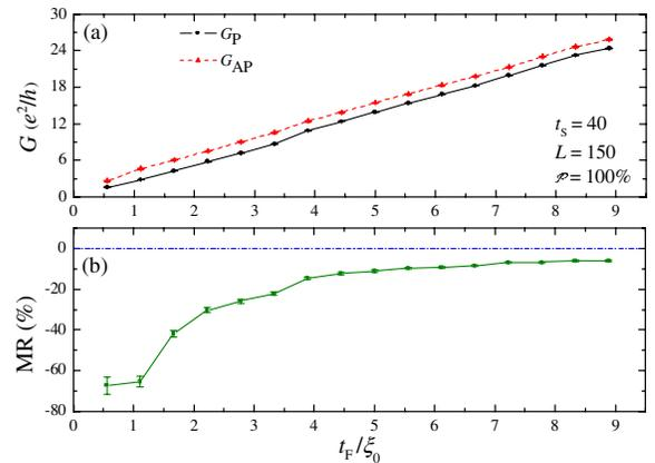
FIG. 3 (color online). (a) Conductance in the  $P$  (black circles) and  $AP$  (red triangles) configurations versus  $t_F$  with  $t_S = 40$ . (b) Resulting MR ratio. The same parameters as for Fig. 2 were used.
