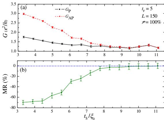
FIG. 2 (color online). (a) Conductance in the  $P$  (black circles) and  $AP$  (red triangles) configurations versus  $t_S$  with  $t_F = 5$ . (b) Resulting MR ratio. Data were obtained assuming  $L = 150$ ,  $\mathcal{P} = 100\%$ , and  $U = 8$  (see text). In (a), the error bars correspond to the standard error over all disorder configurations. Lines are guides to the eye.
