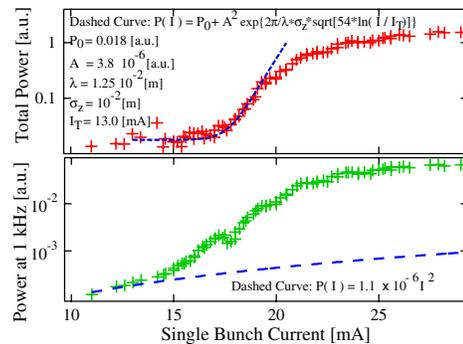
FIG. 3 (color online). Average THz CSR Power versus single bunch current. In the top panel, the measured total power is compared with theory (dashed blue line). In the bottom panel, the CSR power associated with the 1 kHz line of Fig. 2 is compared with the expected quadratic dependence (dashed blue) curve.
