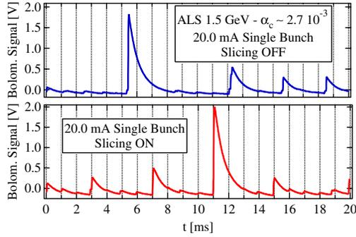
FIG. 1 (color online). Signal induced in a bolometer by the THz CSR bursts associated with the MBI. In the top part the 1 kHz repetition rate slicing laser is off while in the bottom one the laser is on.
