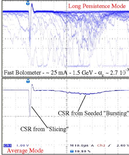
FIG. 4 (color online). The THz CSR signal as measured by a fast (800 kHz bandwidth) detector and an oscilloscope triggered with the 1 kHz slicing signal. In the top panel the oscilloscope is in long persistence mode and many individual laser slicing and burst events are observed. The lower panel shows the averaged detected THz CSR intensity.
