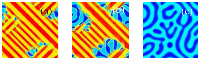
FIG. 3 (color online). Microstructures for x_{12} = x_{1c} = 0 at T = 0.49 and (a) t = 4000 , (b) t = 6000 , and (c) t = 12000 . Red and yellow: martensite; light and dark blue: pearlite.
