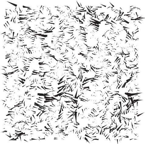
FIG. 1. Inhomogeneous part \delta u(r) of the displacement field u(r) for the imposed macroscopic uniaxial strain in elongation \epsilon_{xx} = 5 \times 10^{-3} for a silica glass containing N = 42000 particles ( L = 83.8 Å). Projection of the field is done on the (x-z) plane for all particles with position r close to the plane. The arrow length is proportional to \delta u(r) and scaled by a factor of 150. The field resides in the linear elastic regime, i.e., has a magnitude varying linearly and reversibly with the applied deformation. As visual inspection shows, it is strongly spatially correlated and involves a substantial fraction of all atoms.
