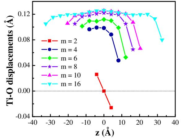
FIG. 3 (color online). Relative Ti-O displacements in a ferroelectric BaTiO<sub>3</sub> film for different  $m$ . Positive values correspond to the local electric dipole moment pointing up as in Fig. 1. The midpoint of the ferroelectric film lies at  $z = 0$ .
