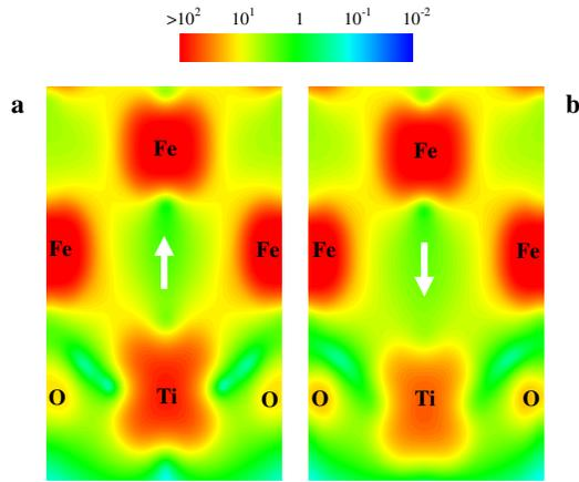
FIG. 4 (color online). Minority-spin charge density (in arbitrary units) at the Fe/BaTiO<sub>3</sub> interface for two opposite polarizations in BaTiO<sub>3</sub>. The charge density is calculated in the energy window from  $E_F - 1$  eV to  $E_F$  in the (010) plane for the  $m = 4$  multilayer. (a) Net polarization pointing up; (b) net polarization pointing down.
