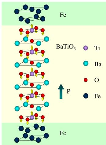
FIG. 1 (color online). Atomic structure of Fe/BaTiO<sub>3</sub> multilayer for  $m = 4$ . Arrows indicate schematically displacements of Ti and O atoms in BaTiO<sub>3</sub> with the net polarization pointing up.
