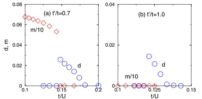
FIG. 4 (color online). Order parameters of the frustrated two-dimensional Hubbard model as a function of pressure (modeled as  $t/U$ ) at zero temperature for (a)  $t'/t = 0.7$  and (b)  $t'/t = 1.0$ .  $d$  (circles) and  $m$  (diamonds) denote the  $d$ -wave SC and AF order parameters, respectively.  $m$  is multiplied by 0.1 to fit in the plots.
