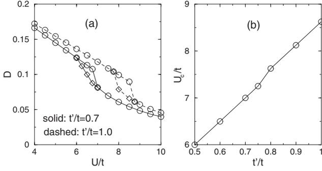
FIG. 2. (a) Double occupancy  $D = \langle n_{\uparrow} n_{\downarrow} \rangle$  as a function of  $U/t$  for  $t'/t = 0.7$  (solid curve) and  $t'/t = 1.0$  (dashed curve); (b) critical  $U_c/t$  as a function of  $t'/t$  in the normal state. The diamond symbols in (a) are obtained with the insulating solution as an initial guess.
