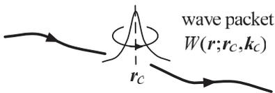
FIG. 1. The wave packet description of a charge carrier whose center is  $(\mathbf{r}_c, \mathbf{k}_c)$ . A wave packet generally possesses two kinds of motion: the center of mass motion and the self-rotation around its center. Both of them contribute to the local current density as given in Eq. (2).
