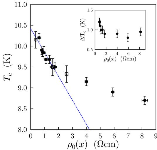
FIG. 4 (color online). The suppression of  $T_c$  compared to the interlayer residual resistivity  $\rho_0(x)$ . The suppression is approximately linear for low damage  $\rho_0(x) < \rho_0^* = 2 \Omega \text{ cm}$ , but there is a change in gradient for  $\rho_0 > \rho_0^*$ . The inset shows the dependence of the width  $\Delta T_c$  of the superconducting transition on  $\rho_0(x)$ . Symbols correspond to those in Fig. 3 and data for an additional undamaged sample are shown by a solid diamond.
