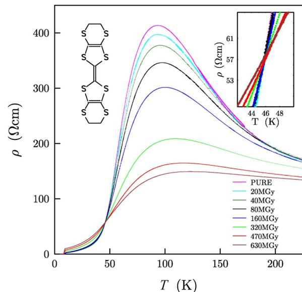
FIG. 1 (color online). Interlayer resistivity of an x-ray damaged sample as a function of temperature for a range of irradiation doses, showing the violation of Matthiessen's rule. Data from the proton-irradiated samples are qualitatively the same. Insets show the ET molecule and a magnified view of the region near  $T_{\text{cross}}$  (defined in the text).
