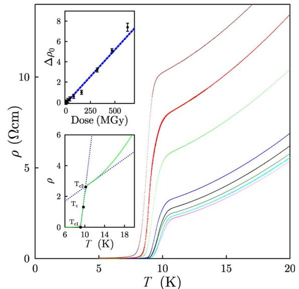
FIG. 2 (color online). The low-temperature region of Fig. 1. The upper inset shows that  $\Delta\rho_0$  increases with x-ray dose in an approximately linear fashion. Data from proton-irradiated samples show a similar pattern as a function of disorder. The lower inset shows three methods of defining the critical temperature: a lower  $T_{c1}$ , an upper  $T_{c2}$ , and  $T_c$ , the maximum of the first derivative, which is the definition used in this Letter.
