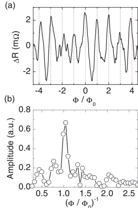
FIG. 3. (a) Magnetoresistance oscillations of the sample shown in Fig. 1(b) measured at  $T = 0.27 \text{ K}$  as a function of a normalized external flux through the loop. Sample resistance is  $94.3 \Omega$ .  $L_F = 120 \text{ nm}$ . (b) Fourier spectrum of the oscillations confirming the  $hc/2e$  periodicity.
