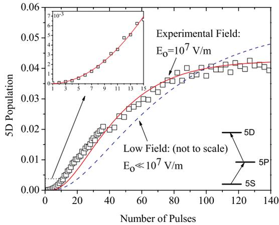
FIG. 2 (color online). The on-resonance  $5D_{5/2}$   $F = 4$  fluorescence signal is measured (squares) at a field strength of  $E_o = 10^7$  V/m vs the number of pulses. The solid (dashed) line is the theoretically predicted excited state populations under experimental (asymptotically low) field strengths. The inset shows the quadratic scaling for the first 15 pulses.
