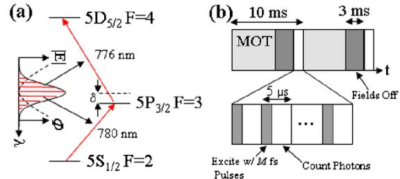
FIG. 1 (color online). (a) Simplified energy level diagram of the three relevant atomic states and frequency domain representation of the chirped comb.  $\delta$  is the detuning of the intermediate state from half the two-photon transition frequency. (b) Timing diagram used in the experiments.
