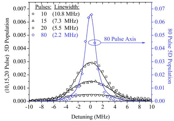
FIG. 3 (color online). The  $5D_{5/2}$   $F = 4$  line shape is measured (symbols) vs the number of applied femtosecond pulses (10, 15, 20, 80 pulses) with the corresponding FWHM linewidth in the legend. The Lorentzian linewidth of 2.2 MHz after 80 pulses is the asymptotic power-broadened linewidth.
