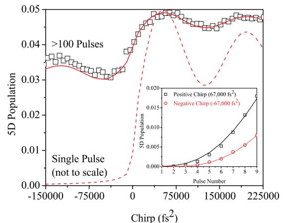
FIG. 4 (color online). The  $5D_{5/2}$   $F = 4$  excited state fluorescence is measured (squares) under steady-state excitation ( $>100$  pulses) vs the applied linear frequency chirp. The solid line indicates the steady-state theory and the dashed line is the single-pulse theory. Inset: the signal (symbols) vs pulse number for two values of equal and opposite chirp; the solid and dashed lines are theoretical predictions.
