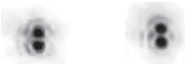
FIG. 3. Two consecutive pictures of a doublet. The quick change ( <1/15 s) is attributed to a switching between two different equilibrium positions which is corroborated by the qualitatively distinct interference patterns. Droplets are \sim 2 \mu\text{m} in diameter.
