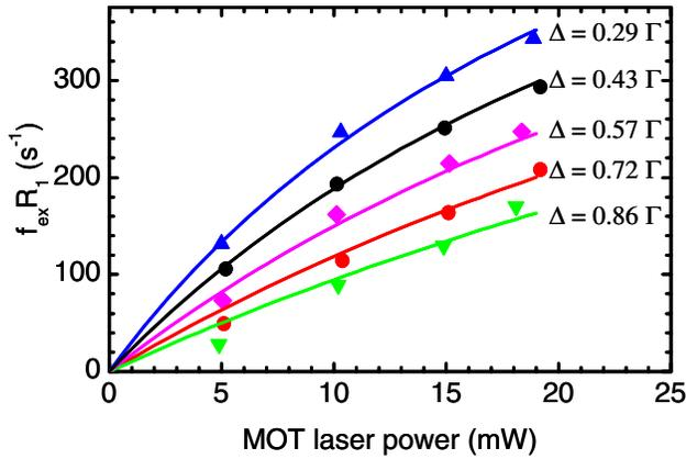
FIG. 3 (color online). Values of  $f_{\text{ex}}R_1$  extracted from the model fit vs MOT power for five different detunings. Symbols indicate experimental values, with uncertainties about the size of the plotting symbols. Solid lines indicate a fit of Eq. (2) to the data. Note that Eq. (2) was fit simultaneously to all detunings and intensities to yield a single set of parameters  $R_1$ ,  $a_1$ , and  $a_2$ .
