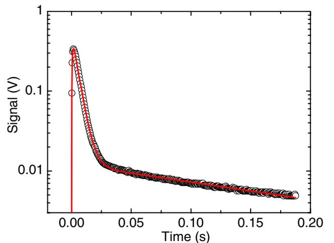
FIG. 2 (color online). Typical time dependence of the MOT fluorescence, beginning when the MOT light is turned on after both the slower and MOT beams have been off for 0.2 s. A clear two-component exponential decay is observed. Experimental values are indicated by open circles, and a fit of the model of Eq. (1) is indicated by a solid line (red online).
