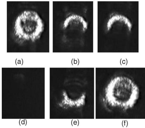
FIG. 3. Diffraction pattern for the electric vector perpendicular to the applied magnetic field in the case of  $3 \mu\text{m}$  magnetic spheres dispersed in a ferrofluid (28% concentration); (b)  $H = 30 \text{ G}$ , (c)  $H = 60 \text{ G}$ , (d)  $H = 100 \text{ G}$ , (e)  $H = 200 \text{ G}$ , (f)  $H = 500 \text{ G}$ . Zero forward scattering is observed for  $H = 100 \text{ G}$  (d).
