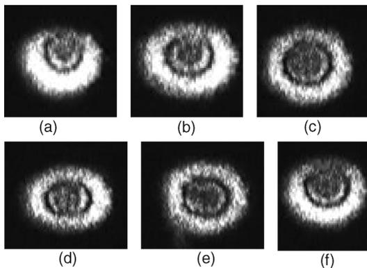
FIG. 4. Diffraction pattern for the electric vector perpendicular to the applied magnetic field in the case of  $2\text{--}3 \mu\text{m}$  silica spheres dispersed in a ferrofluid (28% concentration) (a)  $H = 0 \text{ G}$ , (b)  $H = 30 \text{ G}$ , (c)  $H = 60 \text{ G}$ , (d)  $H = 100 \text{ G}$ , (e)  $H = 200 \text{ G}$ , (f)  $H = 500 \text{ G}$ .
