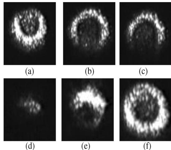
FIG. 2. Diffraction pattern for the electric vector parallel to the applied magnetic field in the case of  $3 \mu\text{m}$  magnetic spheres dispersed in a ferrofluid (28% concentration); (a)  $H = 0 \text{ G}$ , (b)  $H = 30 \text{ G}$ , (c)  $H = 60 \text{ G}$ , (d)  $H = 100 \text{ G}$ , (e)  $H = 200 \text{ G}$ , (f)  $H = 500 \text{ G}$ .
