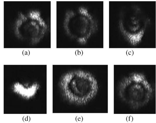
FIG. 5. Diffraction pattern for the electric vector perpendicular to the applied magnetic field in the case of  $3 \mu\text{m}$  magnetic spheres dispersed in kerosene (a)  $H = 0 \text{ G}$ , (b)  $H = 30 \text{ G}$ , (c)  $H = 60 \text{ G}$ , (d)  $H = 100 \text{ G}$ , (e)  $H = 200 \text{ G}$ , (f)  $H = 500 \text{ G}$ .
