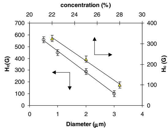
FIG. 6 (color online). Dependency of critical magnetic field ( $H_c$ ) for zero forward scattering on concentration and on the size of the scatterers dispersed in a ferrofluid.
