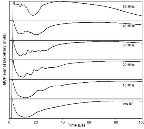
FIG. 1. Typical electron emissions from an expanding ultracold plasma. rf electric fields with the noted frequencies are applied to the expanding plasma, yielding distinct peaks that depend on frequency. The applied rf power is adjusted to make the peaks visible. Note the distortion of the curves at times immediately after the prompt peak for higher rf frequencies, due to the higher rf power required to observe resonance peaks at those frequencies.
