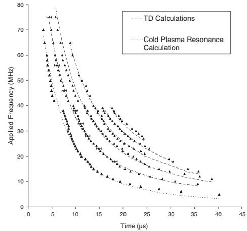
FIG. 2. Mode frequencies vs time. The data have errors at all points approximately the same as the representative error bars. Dashed lines are Tonks-Dattner theory fits with  $T = 19$  K,  $n_0 = 1.9 \times 10^9 \text{ cm}^{-3}$ , and expansion velocity  $v = 65$  m/s. The dotted line is a cold plasma theory fit with  $n_0 = 1.9 \times 10^9 \text{ cm}^{-3}$ ,  $v = 65$  m/s, and multiplicative factor of 0.24 scaling the peak plasma frequency.
