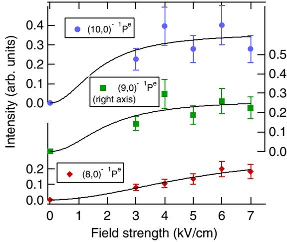
FIG. 3 (color online). Integrated intensities of the Stark induced states labeled 1 in Fig. 2, assigned to the  $(n, 0)^- 1P^e$  series. Solid line: calculated intensity using parameters  $a_n$  (kV/cm) $^2$ : 0.012, 0.029, 0.063 and  $c_n$  (kV/cm) $^2$ : 1, 2.4, 5.4, for the  $n = 8, 9, 10$   $1P^e$  states, respectively. ( $c_n$  has been normalized to 1 for  $n = 8$ ).
