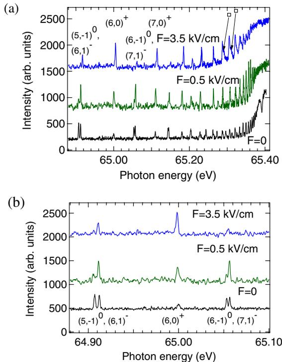
FIG. 1 (color online). (a) Partial fluorescence yield spectra of helium below  $N = 2$  with  $\mathbf{F}$  parallel to  $\mathbf{P}$ . Spectra are normalized to the increase in fluorescence at the  $N = 2$  threshold. (b) Enlarged view of first 5 states.
