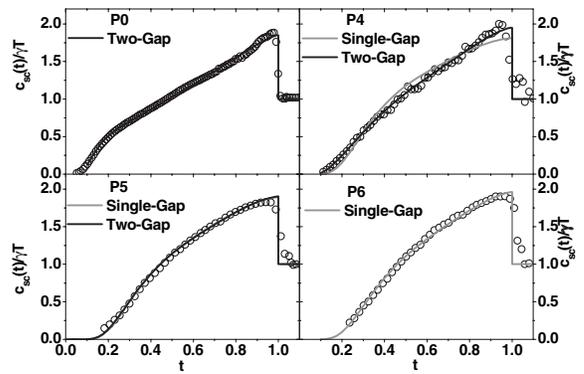
FIG. 3.  $c_{sc}/\gamma T$  as a function of  $t$  for the samples P0, P4, P5, and P6. The best fit curves are plotted as continuous lines. For the samples P4 and P5 the best fit curves obtained within the single-gap (gray line) and two-gap (black line) analyses are presented for comparison.
