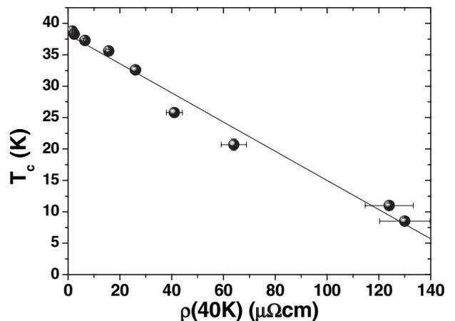
FIG. 1.  $T_c$  versus  $\rho(40)$  for the samples listed in Table I and Ref. [21]. The continuous line is a guide for the eye.
