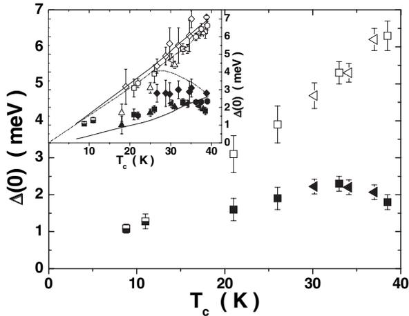
FIG. 4.  $\Delta_{\sigma}(0)$  (empty symbols),  $\Delta_{\pi}(0)$  (filled symbols), and  $\Delta(0)$  (half-filled symbols) as a function of  $T_c$ . In the main figure data from this work (■) and Ref. [19] (◄). In the inset, data from this work (■), Ref. [19] (◄), Ref. [9] (▲), Ref. [16] (►), Ref. [18] (◆), and the theoretical curves calculated in Ref. [7] in the case of only interband scattering (dotted line) and only reduced DOS (continuous line).
