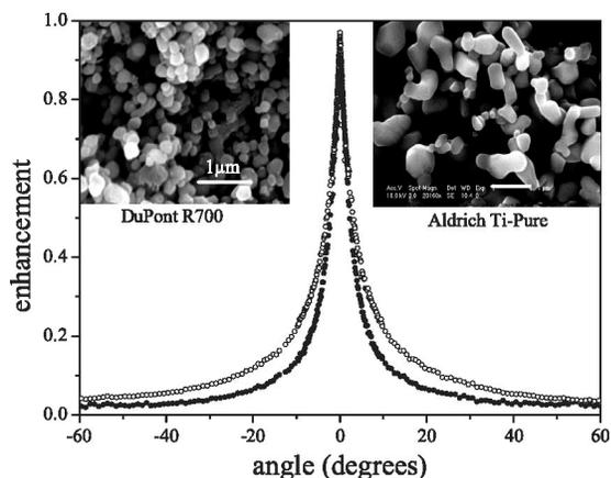
FIG. 1. Measurements of coherent backscattering for two different samples. Open symbols: R700 with an average particle diameter of 250 nm which yields  $k\ell^* = 2.5$ . Closed symbols: Ti-Pure with an average diameter of 540 nm and  $k\ell^* = 6.3$ . All measurements were done with circularly polarized light at a wavelength  $2\pi/k = 590$  nm. The insets show electron micrographs of R700 and Ti-pure.
