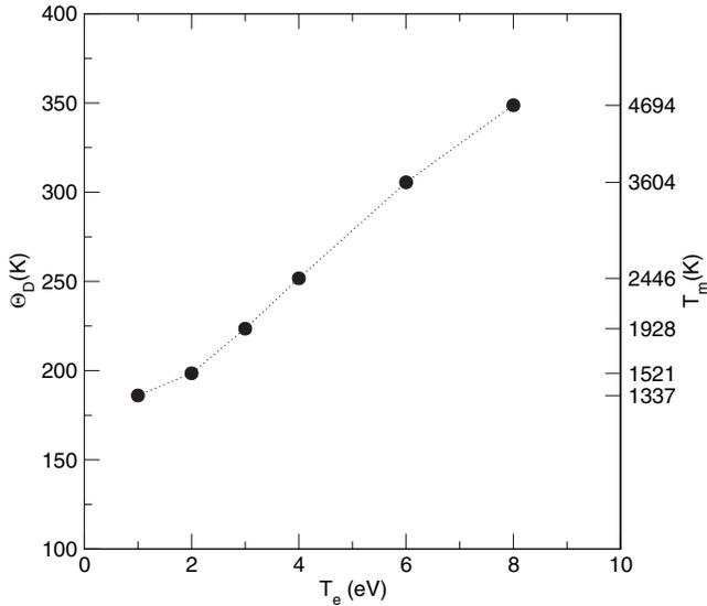
FIG. 3. Debye temperature variation as a function of electronic temperature for gold. On the right-hand side is the corresponding melting temperature.
