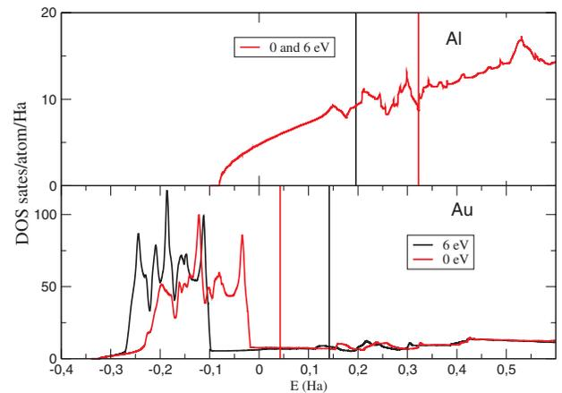
FIG. 4 (color online). Density of state of aluminum and gold at 0 K and 6 eV. Whereas the DOS of aluminum is practically unaffected, the DOS of gold is shifted and shrunk.
