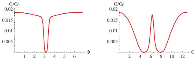
FIG. 3 (color online). Conductance as a function of magnetic field for  $\Phi_2 = 0$  (left panel) and  $\Phi_1 = \Phi_2 = \Phi/2$  (right panel).
