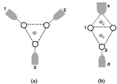
FIG. 1. Triangular triple quantum dot in three-terminal (a) and two-terminal (b) configurations.
