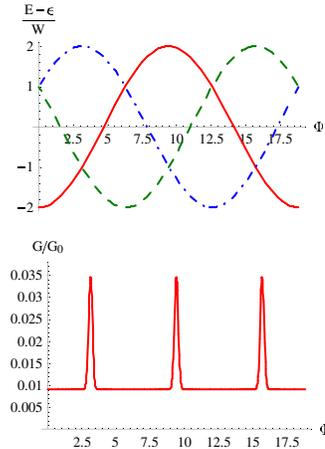
FIG. 2 (color online). Upper panel: Evolution of the energy levels  $E_A$  (solid line) and  $E_\pm$  (dashed and dash-dotted line, respectively). Lower panel: Corresponding evolution of conductance ( $G_0 = \pi e^2/\hbar$ ).
