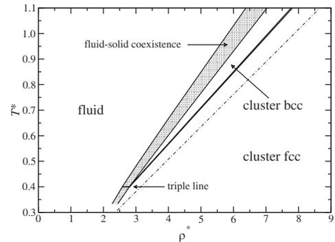
FIG. 1. The phase diagram of the GEM-4 model, as obtained by DFT. The shaded area represents the coexistence region of the liquid and the cluster bcc phase. The dash-dotted curve is the  $\lambda$  line of the system, calculated in the MFA.
