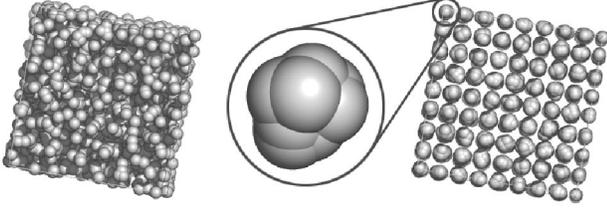
FIG. 2. Two simulation snapshots of a GEM-4 system for  $T^* = 0.4$  and  $\rho^* = 2.5$  and 7 (left and right). The middle panel shows a close-up of one cluster. Particle diameters are not drawn to scale but are chosen to optimize the visibility of the structures.
