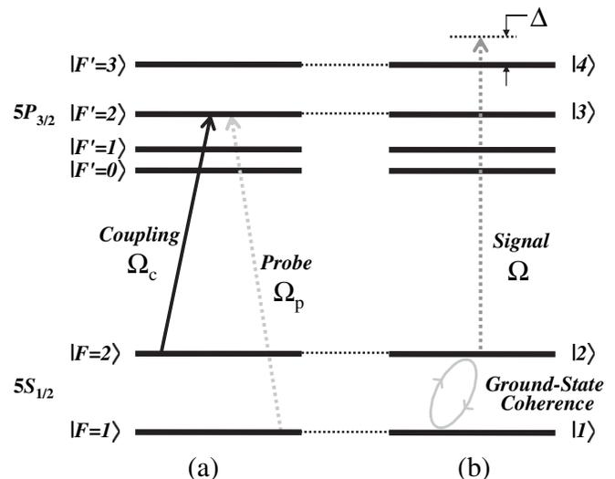
FIG. 1. Relevant energy levels of  $^{87}\text{Rb}$  atoms and laser excitations in the experiment. (a) The coupling and probe fields form the  $\Lambda$ -type EIT configuration. (b) The detuned signal field drives the cycling transition during the light storage.
