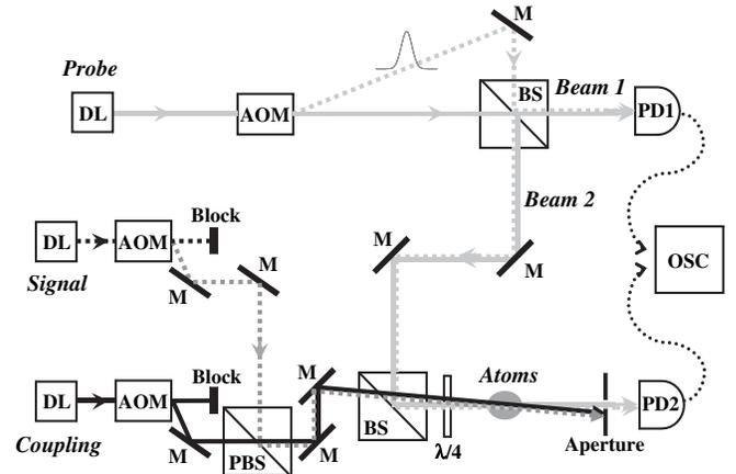
FIG. 2. The experimental setup. DL: diode laser, PD: photodetector, BS: beam splitter cube, PBS: polarizing beam splitter cube,  $\lambda/4$ : quarter wave plate,  $M$ : mirror, OSC: oscilloscope.
